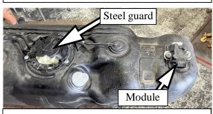
Photo 2: OEM tank preparation
