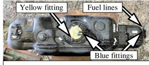
Photo 1: OEM tank preparation
