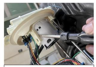
Photo 4: Remove OEM rollover valve
