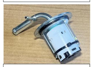
Photo 5: Refit OEM rollover valve
